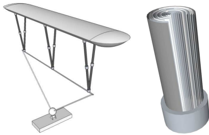
Left: The Wave Harvester with cables made of a stretchable capacitor. Right: Cross section of the capacitor cable.
